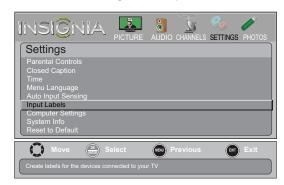
3 Press ▲ or ▼ to highlight Input Labels, then press OK. The Settings-Input Labels screen opens with the input source field highlighted.
